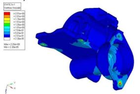
Variation in Von-Mises Stress of Collapsible Steering Column:
