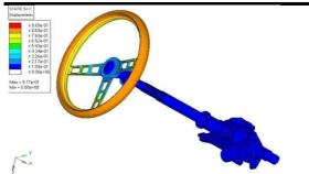
Variation in Von-Mises Stress of Combination Switch Assembly:
